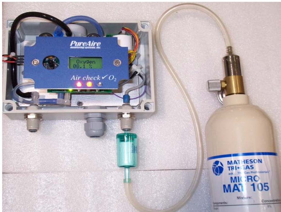
O 2 monitor Connected to gas cylinder
