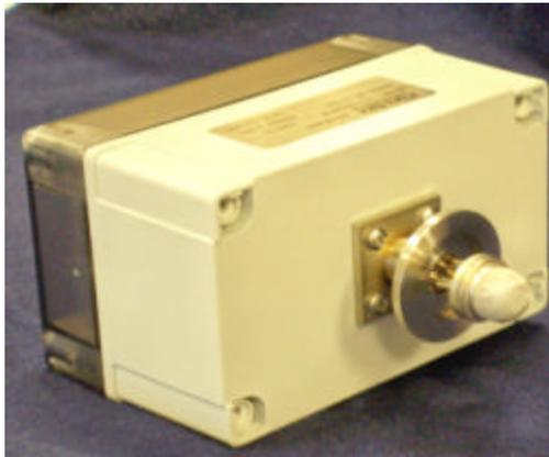
Oxygen monitor with KF flange attached directly to the monitor
