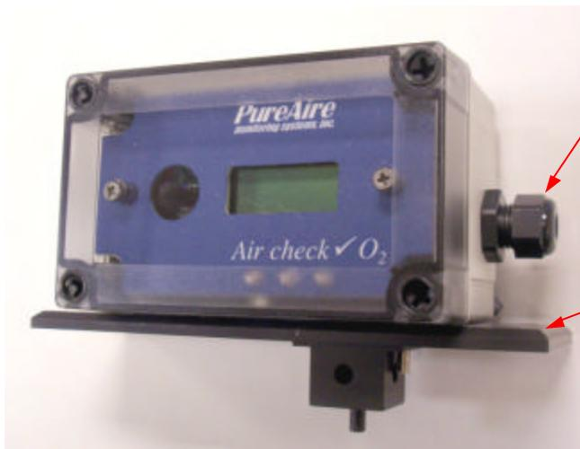
Strain relief for power and relay outputs
