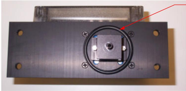
**NOTE:** The O-ring must be installed to insure an airtight seal.
