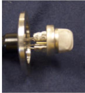
Oxygen cell and KF-25 flange
